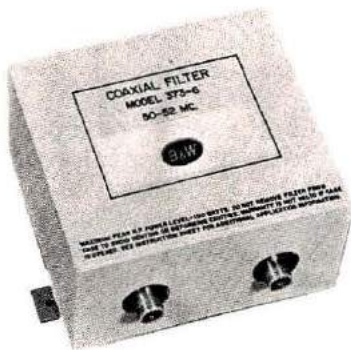
A filter may be necessary to keep transmitter oscillator and multiplier frequencies inside the rig, where they belong. This one, by Barker and Williamson, offers 40 dB of suppression of signals outside its passband, and is rated at 100 watts power handling capability ( photo courtesy Barker and Williamson, Inc. ).
