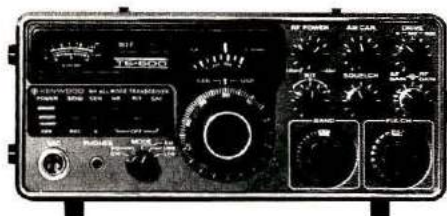
The Kenwood TS-600 transceiver is one of the new breed of multimode rigs designed for six meter, all-mode operation. Similar to its two-meter cousin, it operates on ssb, fm, a-m, or CW. It covers 50 to 54 MHz with a power output of 10 watts (photo courtesy Trio-Kenwood Communications, Inc.).
